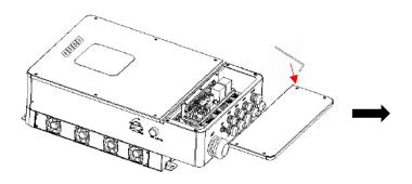
**Step 5**: Pass the corresponding conduit and fasten the joint.
