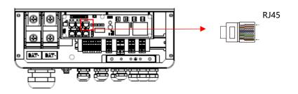
**Step2.** Insert one RJ45 side of the cable into Meter port inside of inverter and the other side into BMS-485port of the meter.
