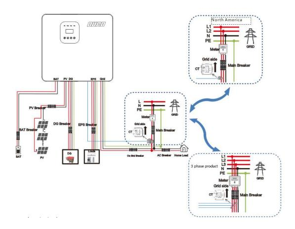
Note: The wiring requirements should be installed as shown in the figure above, Note that the CT crosses the L line, the CT current transformer Arrow marks point to power GRID, RJ45 is connected to "Grid Current" in COM. If it is 3 phase products, will be 3pcs CT crosses to "L1, L2, L3" line.
